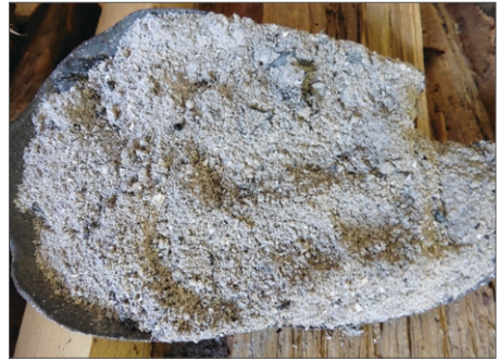
Ashes have a fine structure and are an excellent humidity and odour absorber
