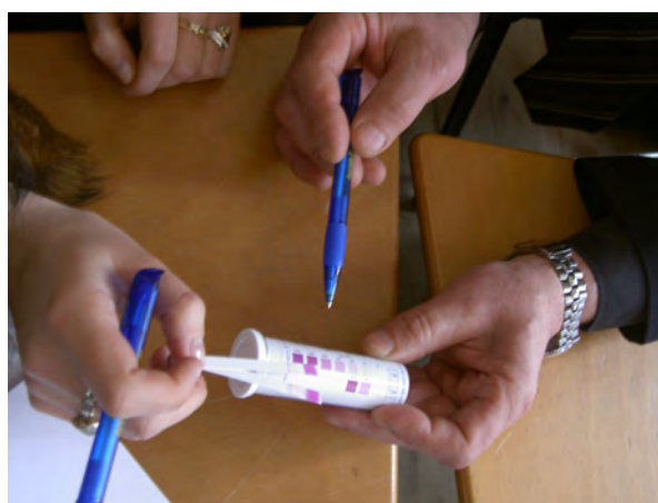
Nitrate test strips are cheap and water samples are quick to analyse
