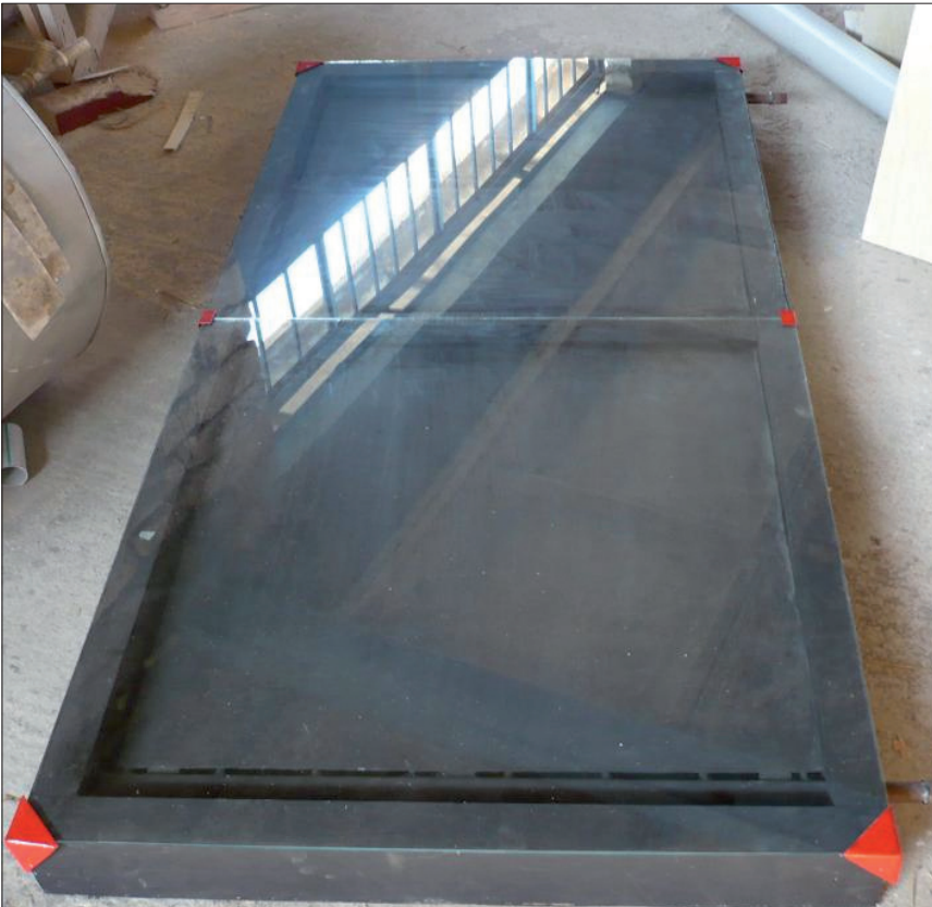
A finished collector
