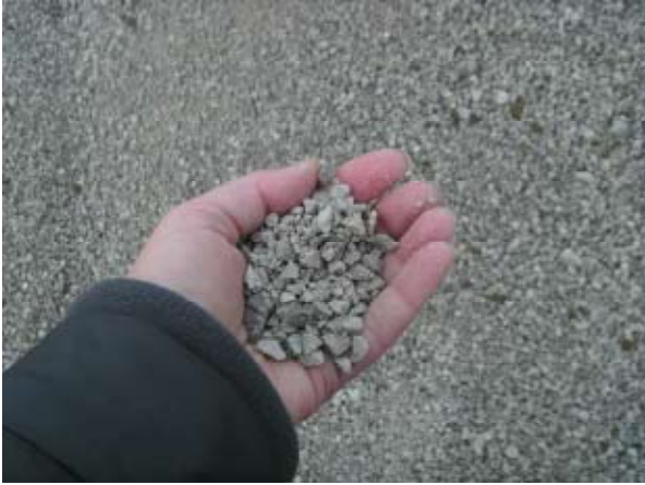
Gravel for drainage layer
