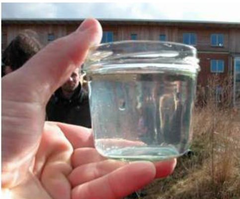
Treated effluent of a constructed wetland
