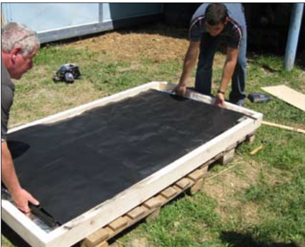
Step 11. Install the absorber into the frame
