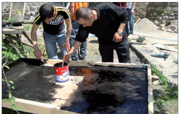
Step 5. Cover the upper part of the frame with plywood, paint black
