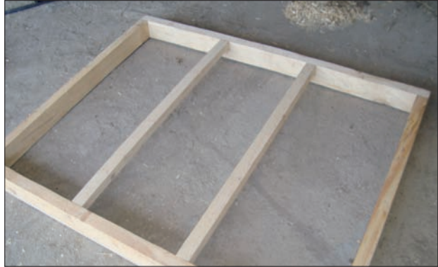
Step 2. Fasten collector bottom and sides
