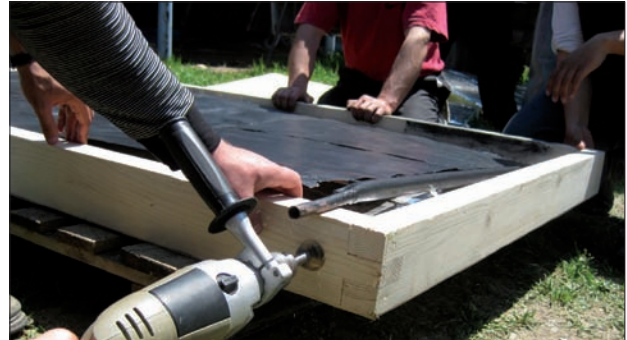
Step 10. Drill inlet, outlet and ventilation holes
