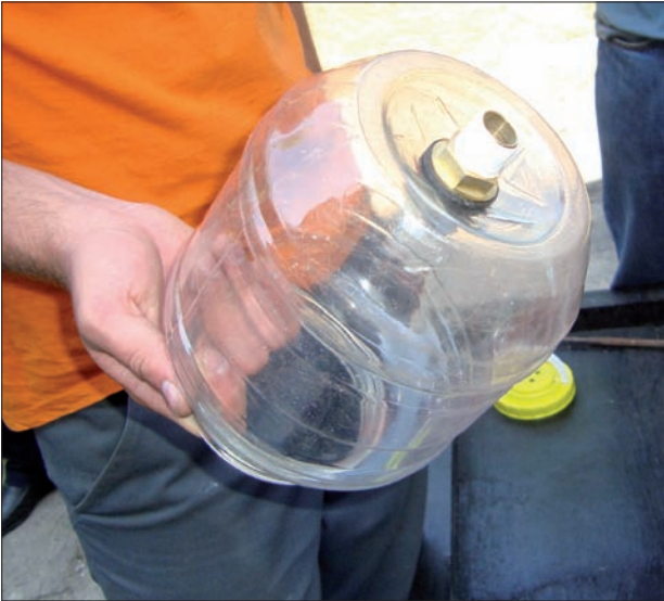
Step 5. Install expansion tank
