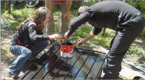
Step 9. Cover with black matt paint or solar lacquer the absorber from both sides
