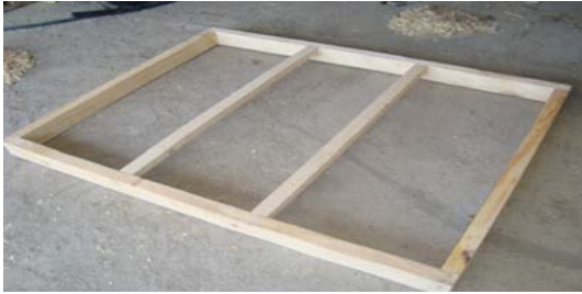
Step 3. Fasten collector bottom and sides
