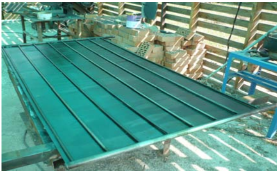
Step 11. Weld to each other the metal tin and the pipes
