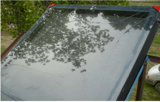
Step 14. Cover the frame with 4 mm thick glass using special metal bars or silicon glue
