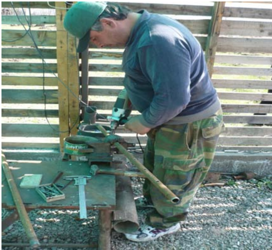
Step 9. Drill 8 holes 12 mm in \frac{3}{4} metal pipes at a distance of 11 cm
