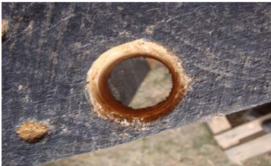
Step 5. Drill inlet, outlet and vent holes
