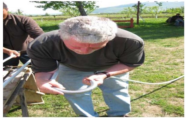
Step 10. Make the serpentine from plastic pipe
