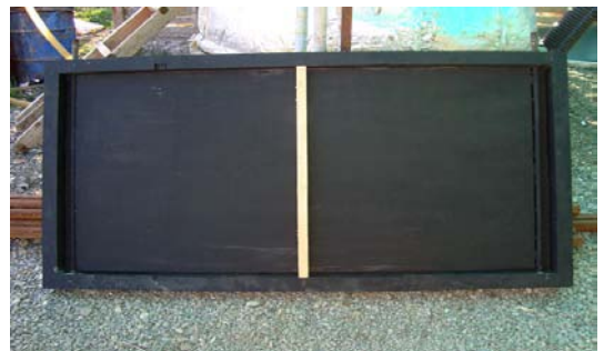
Step 8. Cover the frame and upper part with black matt paint
