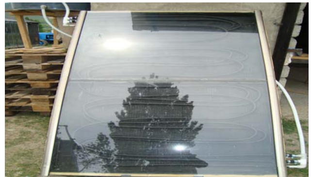
Step 12. Cover the frame with 4 mm thick glass using special metal bars or silicon glue
