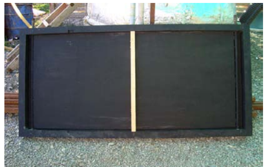
Step 8. Cover the frame and upper part with black matt paint
