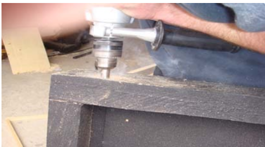
Step 5. Drill inlet, outlet and vent holes
