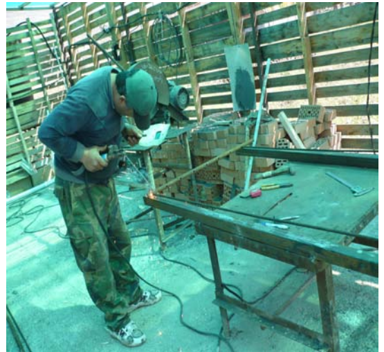
Step 10. Weld the \frac{1}{2} mm pipes to \frac{3}{4} pipes
