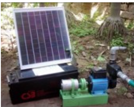
Solar water pump
